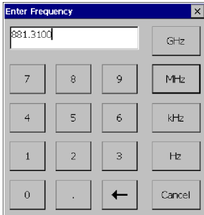
Figure 3-32: Entering the measurement frequency with the keypad
